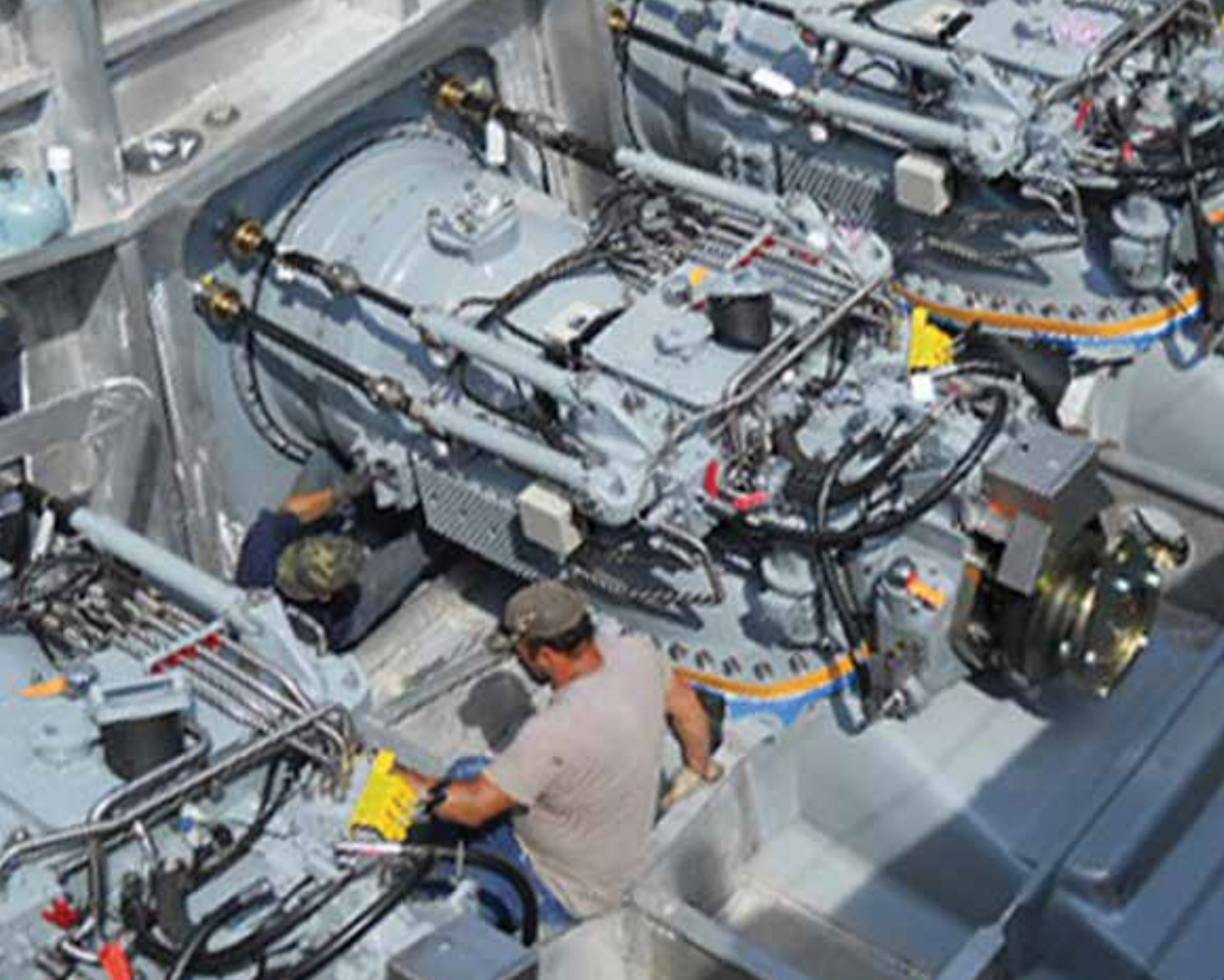
Above and Below: Crewboat "Aaron McCall" was the first vessel to be fitted with quadruple HamiltonJet HT900 waterjets
